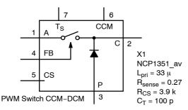
Figure 9. The PWM Switch Encapsulated into a Sub Circuit
