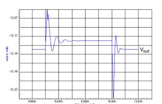
Scale: Y = 20 mV / div, X = 1 ms / div Figure 13. Simulated Load Step Response
