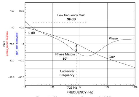
Figure 19. Measured Loop Response in DCM
