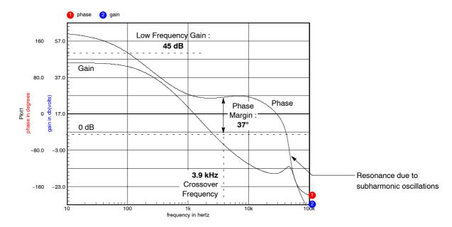
Figure 17. Simulated Loop Response in CCM
