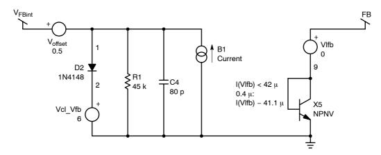
Figure 7. Feedback Modulator Model
