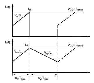
Figure 5. The Current Waveforms in CCM: Ia, Ic
