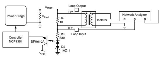
Figure 15. Loop Response Measurement Principle
