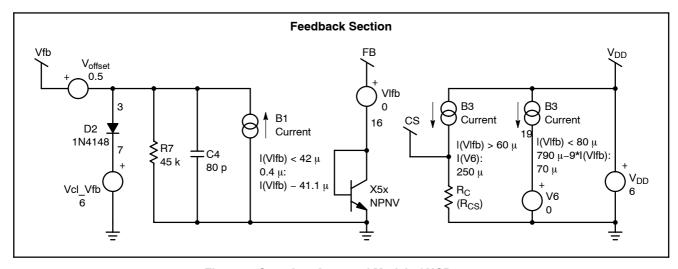
Figure 8. Complete Averaged Model of NCP1351
