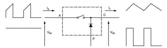
Figure 1. PWM Switch and its Variables
