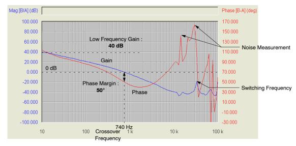
Figure 18. Measured Loop Response in CCM
