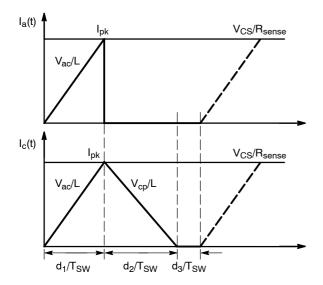
Figure 4. The Current Waveforms in DCM: Ia, Ic
