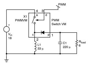
Figure 3. PWM Switch in the Buck-boost Converter
