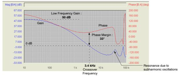
Figure 16. Measured Loop Response in CCM
