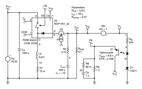
Figure 12. The Buck-boost Model Implemented in SPICE
