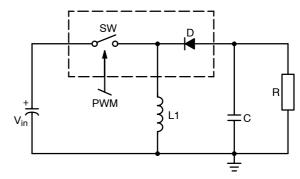
Figure 2. Buck-Boost Converter
