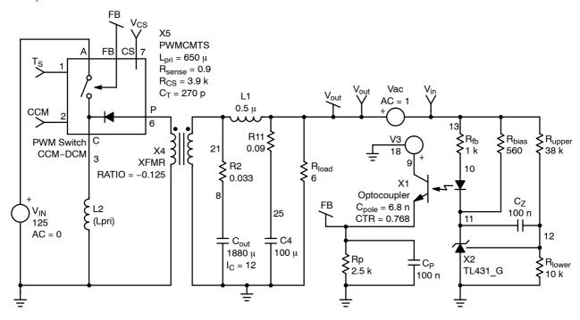
Figure 10. The NCP1351 Model in a Flyback Converter
